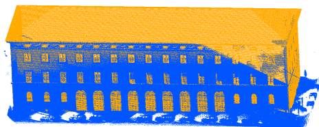
Figure 6. Manual registration result. Target: orange, model point cloud; Source: blue, thermal point cloud.
