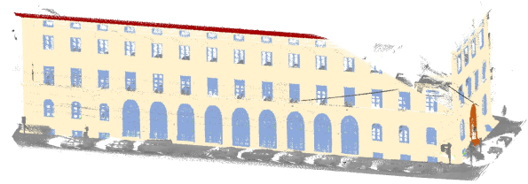
Figure 7. Semantically enriched thermal point clouds.
