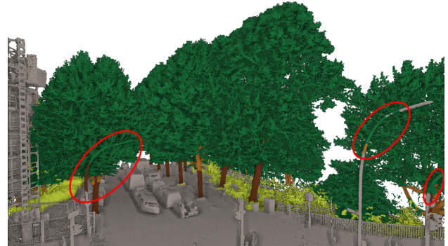
Figure 3. Results of the DL semantic segmentation approach for the 3D point cloud HAG1. Segmentation errors are marked in red.
