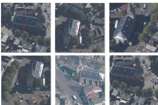
Figure 4. Optimal image selection for facade texture mapping
