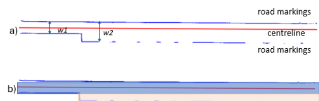
Figure 3. a) Input data (road width: w1 , w2 , centreline, road markings) to delineate road space. b) driving lane with blue colour, parking area with pink colour.
