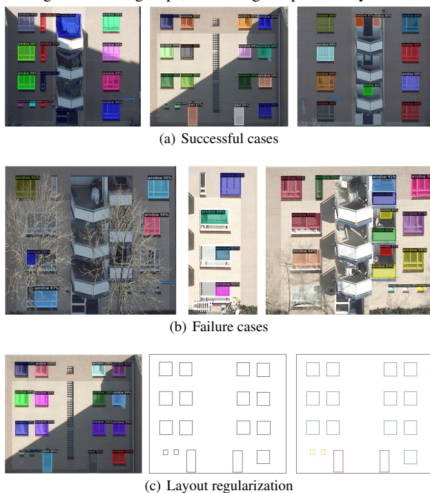
Figure 10. Mask R-CNN façade opening detection results.
