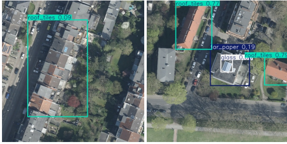
Figure 4. Example cases where a segmented roof may contain multiple buildings (left), and vice versa, where a building may contain multiple detected roofs (right).
