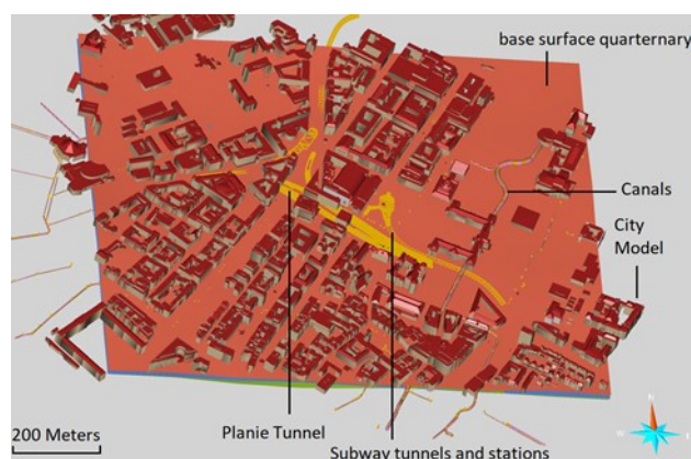
Figure 3. Location of infrastructure components, as described in section 3.2, within the Quaternary horizon (red) of the study area.
