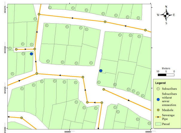
Figure 3. Visualization of selected unconnected subscribers alongside the existing sewer network and parcel boundaries.
