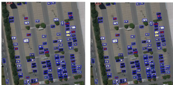
Figure 2. Comparison of vehicle detection results for YOLO models with pre-trained models on MS-COCO dataset, tested on the EAGLE dataset: (a) YOLO12-n, (b) YOLO12-m. Red bounding boxes: false positives, blue: false negatives, green: true positives.
