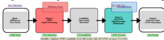
Figure 6. The hybrid screening and refinement pipeline. Stage 1: Fast STPD triage screens all time series, flagging ~5% as candidates. Stage 2: High-precision ATGLSTM refines only the candidates. This combines STPD's scalability (0.2s/1000 series) with ATGLSTM's accuracy ( F1 \approx 0.75-0.80 ) for efficient, large-scale processing.
