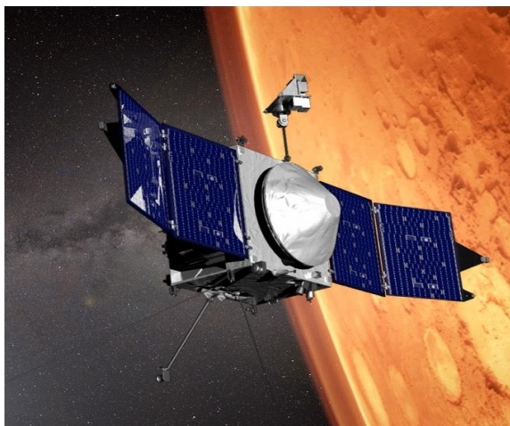
Figure 1. Mars Atmosphere and Volatile Evolution (MAVEN) spacecraft is developed and operated by NASA in 2013. Since entering Martian orbit in 2014, MAVEN has been studying the planet's upper atmosphere, ionosphere, and interactions with the solar wind. Equipped with instruments such as the Solar Wind Electron Analyzer (SWEA), the Langmuir Probe and Waves (LPW) system, and the Magnetometer (MAG), the spacecraft provides in-situ measurements that are critical for understanding Mars' plasma environment and atmospheric escape processes.
