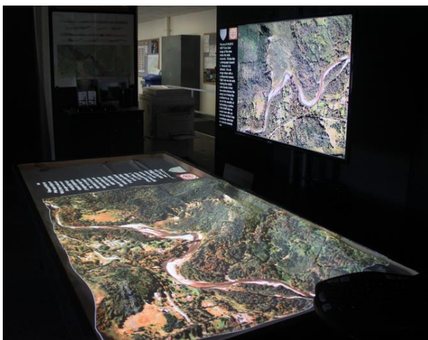
Figure 4. ARES AR sandbox with pre-landslide aerial imagery of the Oso region projected on the sculpted sand surface.
