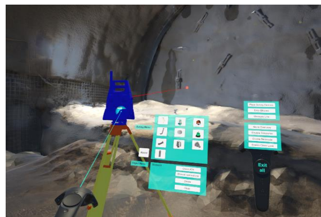
Figure 3. Simulation of a total station in a tunneling scenario.
