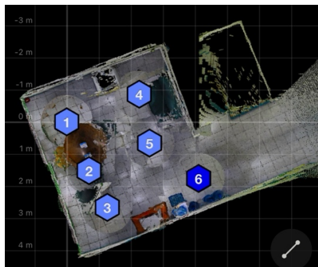
Figure 10. 3D scans oriented and aligned in Matterport
