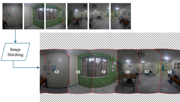
Figure 2. Stitching raw images to form omnidirectional images
