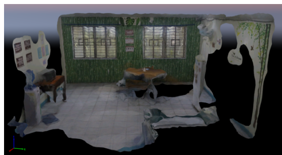
Figure 9. Mesh generated from the desktop-based platform using omnidirectional images
