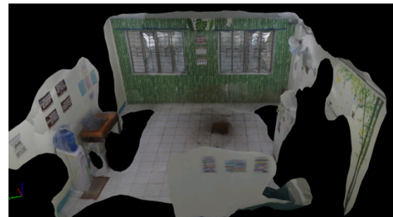
Figure 7. Mesh generated from the image capture method suggested by Pix4D best practices
