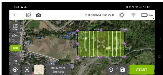
Figure 4. Flight plan conducted by participants in New Washington, Aklan to demonstrate execution of autonomous flight planning.
