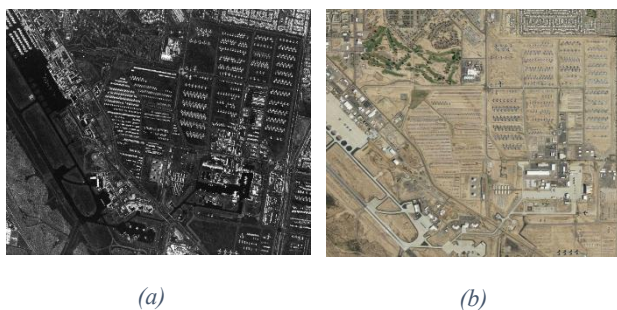
Figure 1: (a) SAR image acquired from Airbus TanDEM-X mission (Spotlight mode) © Airbus DS 2025 (b) Optical image obtained from Google Earth Pro © Google Earth, Landsat/Copernicus, 2025.
