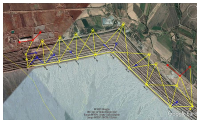
Figure 4. Layout of working benchmarks located on the dam and the adjacent area
