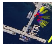
Figure 10. Zamboanga's Fresnel Zone and Ideal Location for GNSS-IR Station (yellow arrow)
