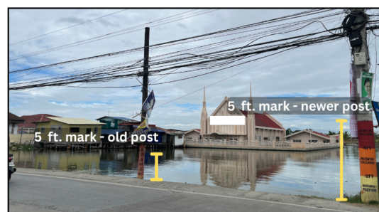
Figure 7. Comparison of height references between an old and newer post in Hagonoy, Bulacan, showing deeper ground embedding of the older post based on 5-ft. marks.
