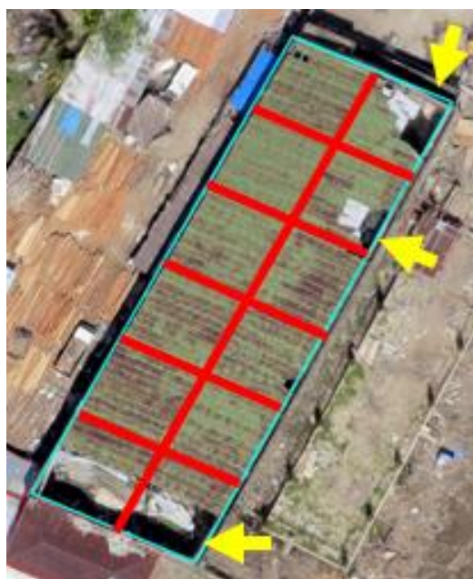
Figure 3. Building with damage rating of 2. Yellow arrows show the damage indicators. Damaged area is approximately less than 20 percent of the total building polygon's area.
