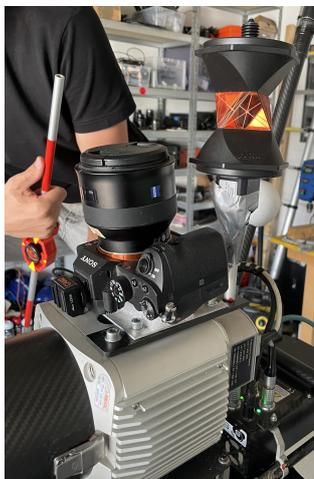
Figure 2. Rigid mounting of a) 360° prism, b) RIEGL VUX-SYS including Applanix AP-20 and c) Sony Alpha 7R II on our UAS
