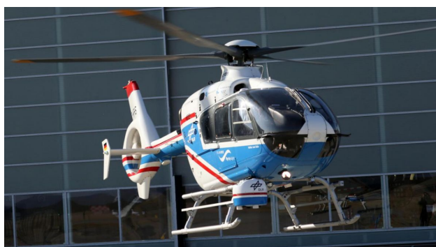
Figure 2. VABENE camera system mounted on DLR's research helicopter D-HFHS.
