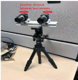
Figure 10. Camera Setup and Imaging Geometry.
