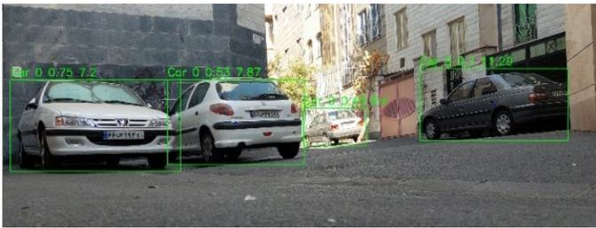
Figure 13. The image captured by the left camera includes annotations for each class, indicating the confidence percentage and the distance to each detected object.
