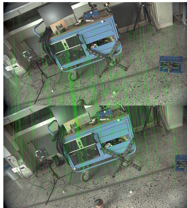
Figure 7. Two pictures with the corresponding tie point matches
