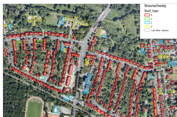
Figure 1. Classification results of BEit model pretrained using Aerial Image Dataset on building roof types in the Braunschweig area.
