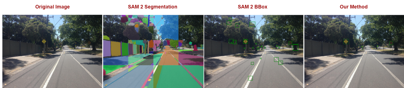
Figure 3: Comparison of segmentation results between SAM 2 (Ravi et al., 2024) and our Domain-Specific Agnostic Segmentation with Contrastive Learning method (see Figure 1(a)). SAM 2 tends to over-segment, including irrelevant objects like traffic signs. Our method, by focusing on city-specific contrastive learning and fine-tuning, avoids this issue and achieves more accurate transit sign detection.
