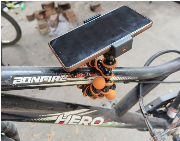
Figure 1 : Setup of the smartphone on crossbar of the bicycle.
