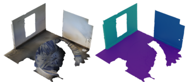
Figure 3. Left, an indoor scene where the detected objects have been removed. Right, the 3 detected planes from the RANSAC algorithm.
