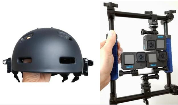
**Figure 5.** The POC Crane Mips helmet onto which the three cameras can be mounted (left); Three GoPro cameras mounted inside a frame composed of standard camera rig components (right).
