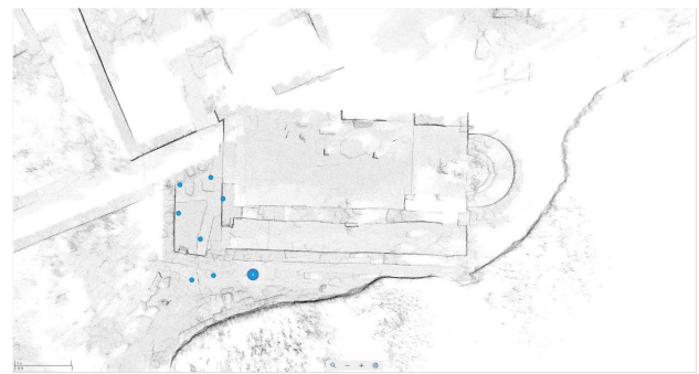
Figure 14. Layout of scan cluster for the excavation at the narthex of the Basilica of Agios Kirykos, Delos.
