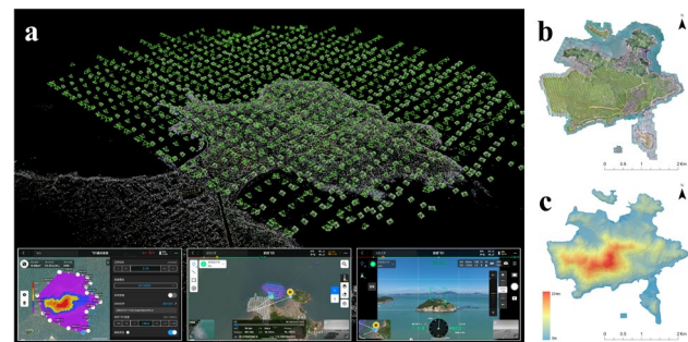
Figure 12. (a) RTK drones oblique photography. (b) Orthophotos. (c) Digital surface models.
