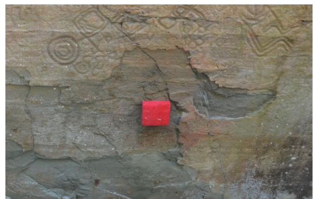
Figure 6. Attaching a test specimen for the assumption of damaged conditions.
