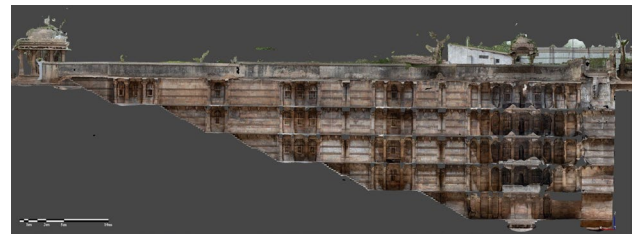
Figure 1. Section of Bai Harir Ni Vav Stepwell, Ahmedabad generated through photogrammetry documentation.
