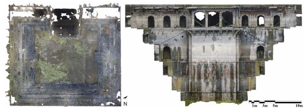
Figure 2. Site plan and section of Modi Ka Chopda, Jhansi, generated through photogrammetry documentation
