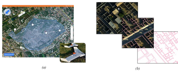
Figure 6. Survey plan for the acquisition of orthophotos of the Park via drone
