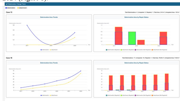
Figure 10. Retrieval results of caves with deterioration and detachment without restoration.
