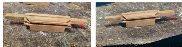
Figure 9. Half-Tenon Joint (Photograph on the Left, Point Cloud Data on the Right)
