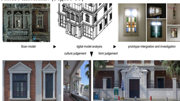
Figure 11. Design judgement according to HBIM model, history material, and prototype analysis.
