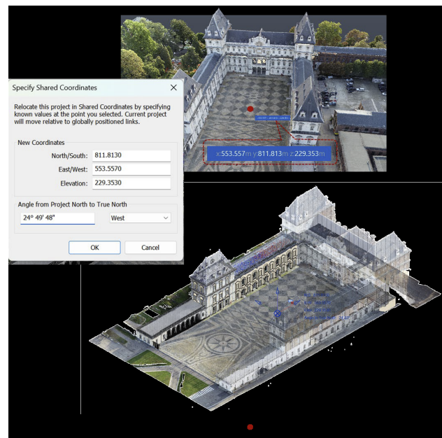
Figure 3. Definition of the Project Base Point.
