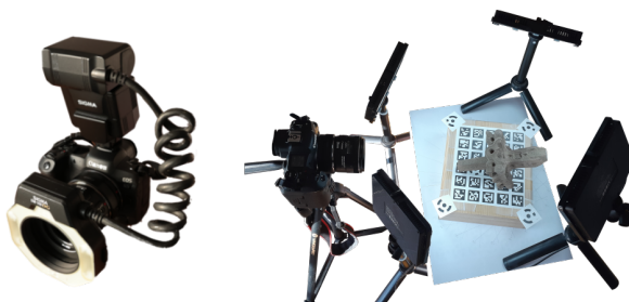
Figure 5. Equipment for both photographic acquisitions. On the left, with ring flash for on-the-fly shots. On the right, focus-stacking-ready setup.
