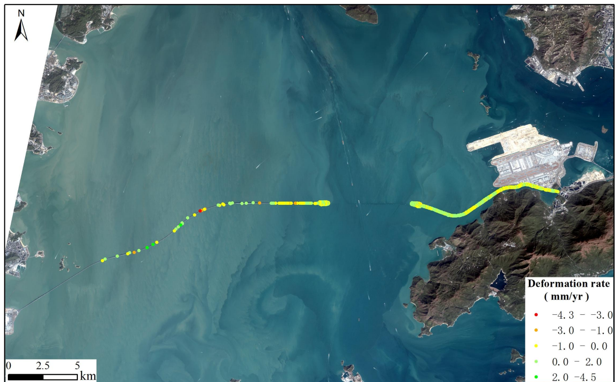
Figure 2. The SBAS results of the HZMB from the LT-1 descending orbit overlaid on a ZY-3 optical image.
