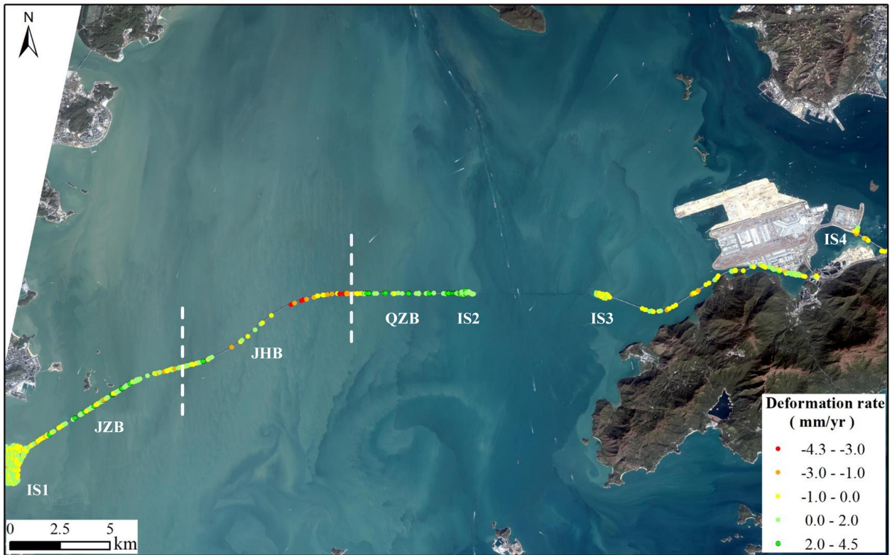
Figure 1. The SBAS results of the HZMB from the LT-1 ascending orbit overlaid on a ZY-3 optical image.
