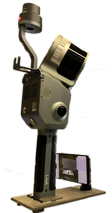
Figure 1. Handheld Lixel L2 Pro laser scanner with fixed mounted camera.
