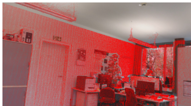
Figure 9. The point cloud shown in Figure 7 was projected onto the image plane.
