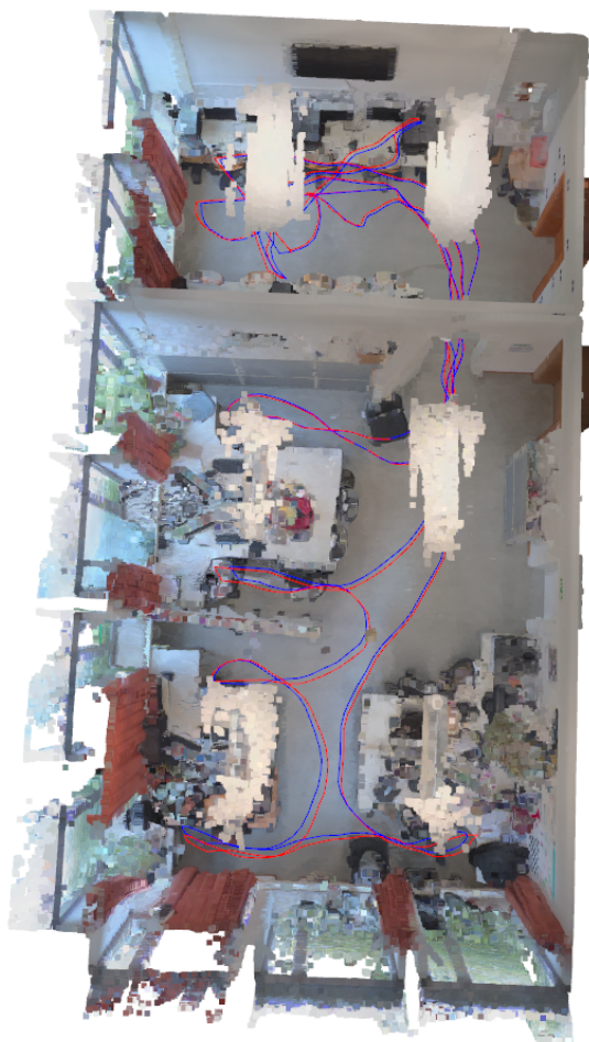
Figure 8. Visualization of movement trajectories. The trajectory of the smartphone was determined using the method presented here and is shown in blue, while the trajectory of the smartphone determined using photogrammetry is shown in red.
