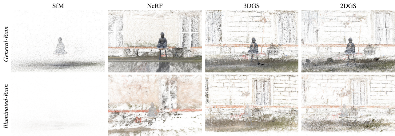
Figure 3. Point cloud reconstruction for both rainy scenarios. Due to its dynamic nature the rain is not reconstructed in the scene, but impacts the geometry of the features it occludes.
