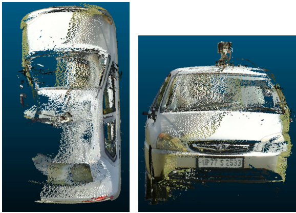
Figure 11. Top view (left) and front view (right) of the car after applying the motion correction algorithm.
