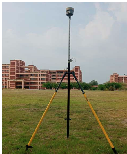
Figure 4. GCPs are setup using Trimble R10 GNSS receiver. GNSS observation is recorded for at least 30 minutes at each GCP.
