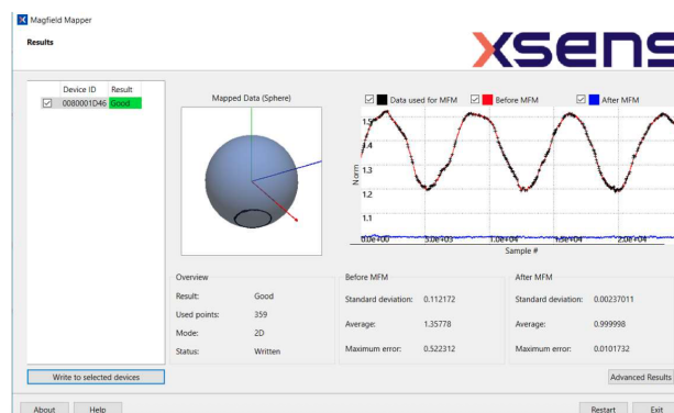
Figure 7. Magnetic field mapper software for calibration of Xsens MTi-680G.
