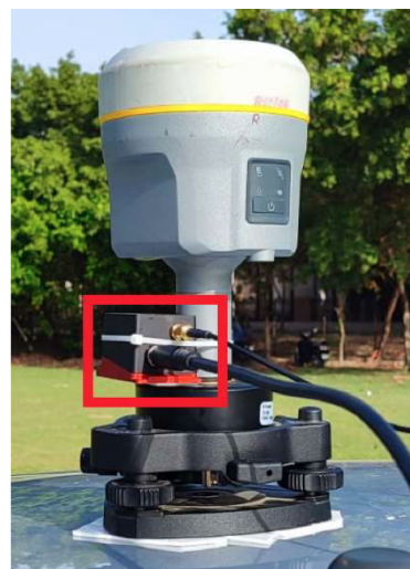
Figure 2. Xsens Mti-680G and Trimble R10 installed on top of the moving car, on a tribrach. The INS of Xsens system is marked with a red square.
