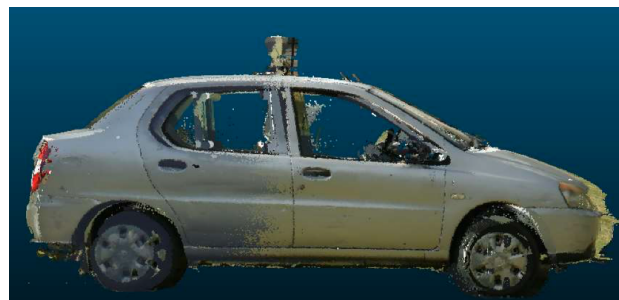
Figure 10. Side view of the car after applying the motion correction algorithm.
