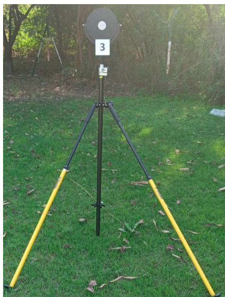
Figure 5. A circular target plate is installed at each of the GCPs. The identification of each GCP is mentioned alongside the target
