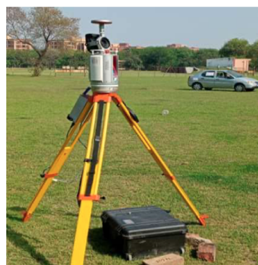
Figure 3. REIGL VZ-2000i TLS used for validation of motion correction algorithm, with the moving object (car) seen in the background.
