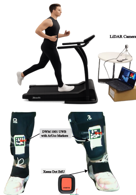
Figure 2. Subject is equipped with DWM1001 UWB sensors with ArUco Markers attached on top of them. Xsens DOT IMU is placed on the heel of the left foot. Ground truth is collected using the Intel Realsense LiDAR Camera.
