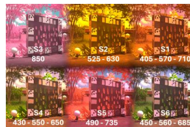
Figure 1 – The six sub-images (S1, S2, ..., S6) of the multispectral Agrowing camera and the respective wavelengths (in nm) for each sub-image.
