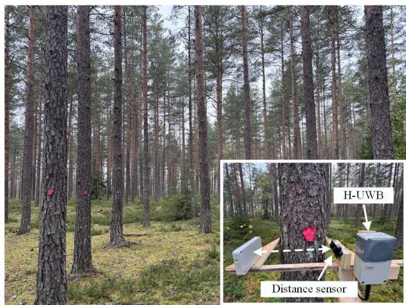
Figure 1. Overview of the forest plot used in this study and the developed prototype of the integrated heading and UWB device (H-UWB), equipped with an ultrasonic distance sensor for real-time DBH measurement and position correction.
