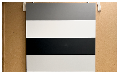
Figure 1. Target for the determination of the angular precision. Target size \approx 100 \times 100 cm.
