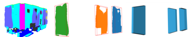
Figure 3: From left to right: the result of semantic segmentation using PTV1, the bounding box results after clustering using DBSCAN and the IFC output for window detection for Office 1 Area 5 of S3DIS Dataset
