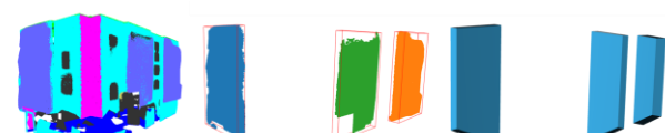
Figure 4: From left to right: the result of semantic segmentation using PTV3, the bounding box results after clustering using DBSCAN and the IFC output for window detection for Office 1 Area 5 of S3DIS Dataset
