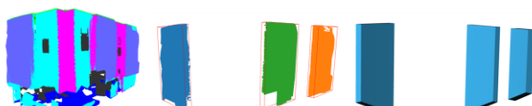
Figure 5: From left to right: the result of semantic segmentation using Swin3D, the bounding box results after clustering using DBSCAN and the IFC output for window detection for Office 1 Area 5 of S3DIS Dataset
