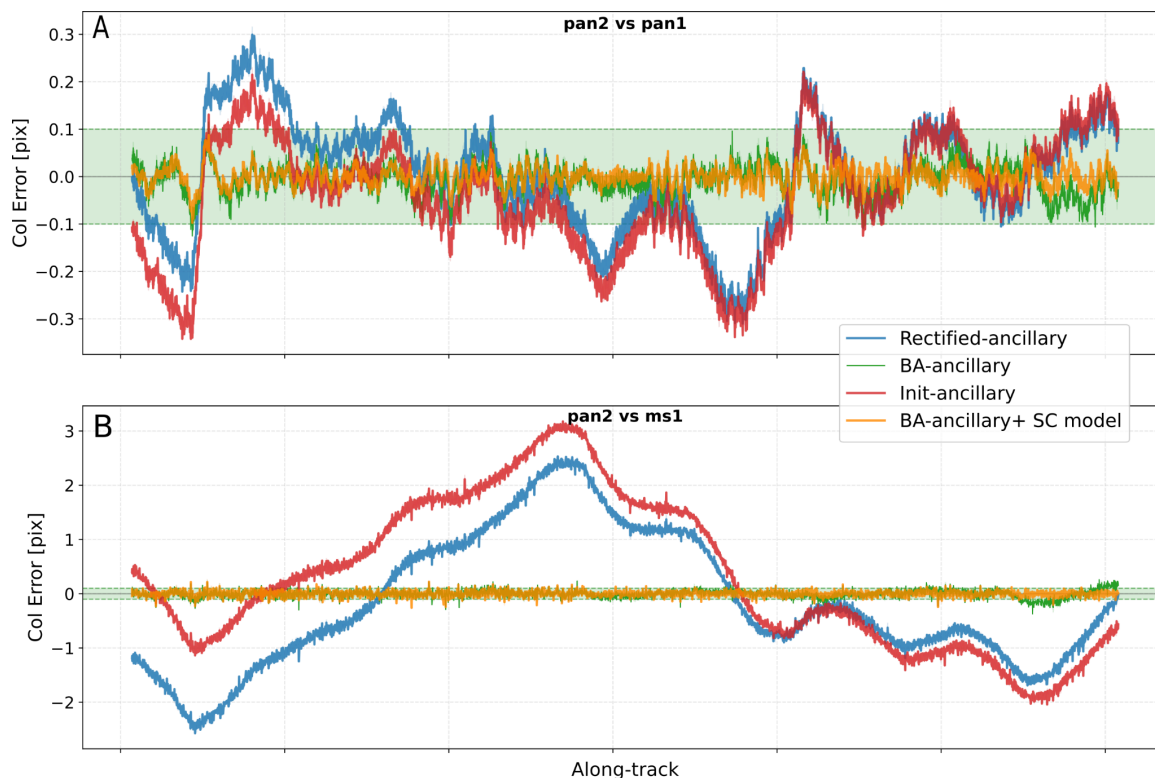
Figure 3. Band-to-band registration error across the four processing phases. Panel (A) shows the along-track error between the PAN1-PAN2 band pair, while Panel (B) presents the along-track error between PAN2-MS1.
