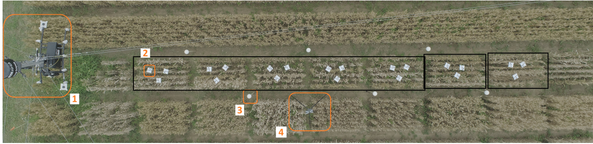
Figure 3. Overview of experiment setup and data collection. Orange rectangles: (1) field phenotyping platform with a camera rig, (2) photogrammetric target (coded marker), (3) reference sphere, (4) TLS. Black rectangles: 7 wheat plots covered within a measurement campaign, from left to right - 5 training, 1 validation, 1 test / hold-out plot.
