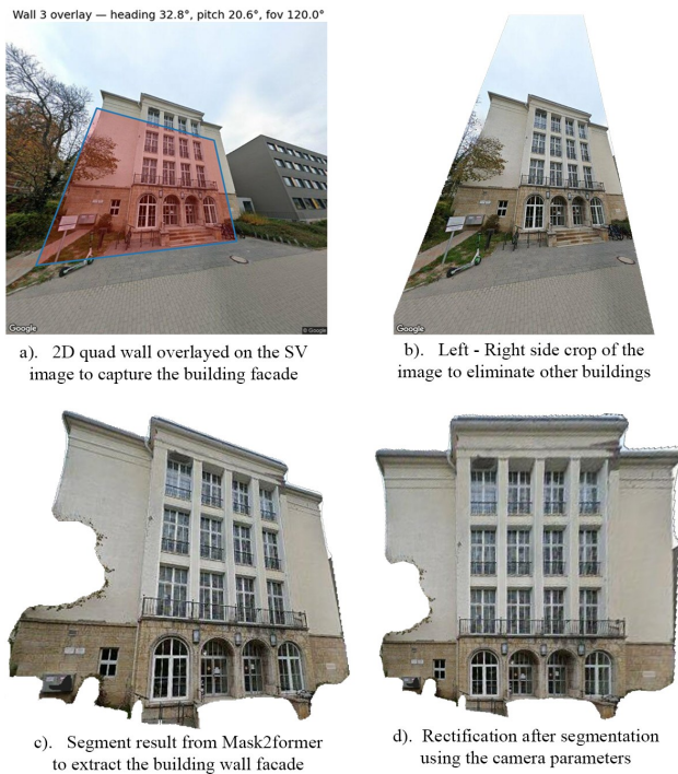
Figure 6. Wall facade generation from a) GSV image using b) cropping, c) segmentation and d) rectification.
